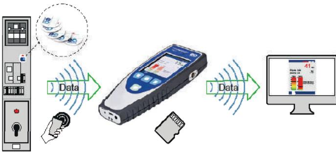
The UltraTEV Plus<sup>2</sup> has NFC capability to store Asset data on programmable tags. It also has the ability to transfer the results directly on to your PC via Wifi or USB / SD Card. The survey functionality allows details of substations and assets to be entered on the screen, guiding users through the simple survey process. Screen shots can also be captured and saved.
