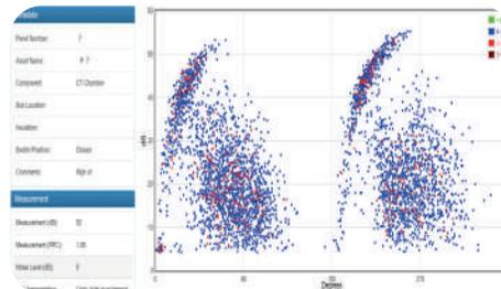
Example of internal void PD measured using the TEV sensor. Asset information can be transferred and sent to EA Technology or your in house PD experts for review.
