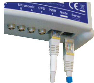
Figure 3: Details of Node Ethernet cable colour coding
