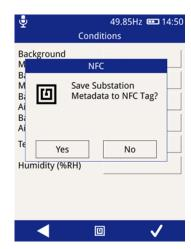
In future, any time a technician comes into the substation to start a survey, this NFC Asset Tag can be read with the UltraTEV Plus2 and this information will be populated into the new survey instantly and accurately.
