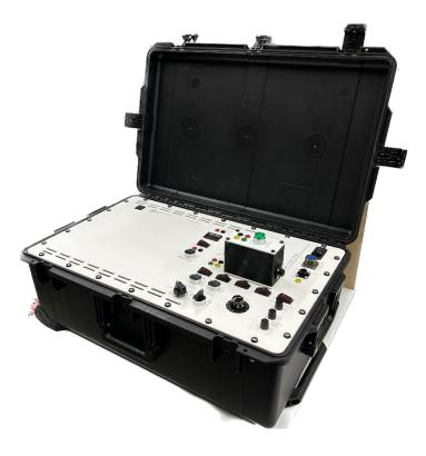
The VDPRG-V4 test set is designed for use by qualified electrical testing personnel, and helps the user perform the Z32 tests in Health Care environments with one comprehensive system. Saves time and improves efficiency of the testing procedures.
