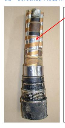
1. Note the only difference from normal PILCSWA is the presence of aluminium foil or copper tapes around each phase conductor's semiconducting layer.
