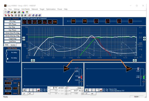
Fig.22 Hybrid - Passive/Active Digital Speaker with DSP. The amplifier(s) are combined by using one only (shown w orange line)
