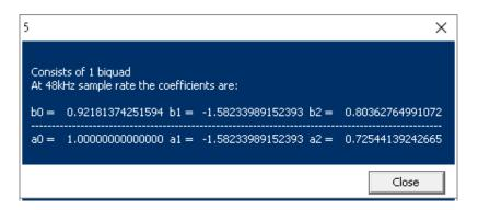
Fig.9 Biquad Coefficients for the 3133Hz Peak/Dip filter
