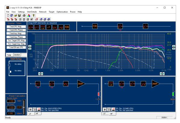
Fig.11 Advanced 2-way example with 15-30-45 degree off-axis responses. The 30deg curve (White) was optimized. The resulting Phase Response is shown as a dashed white line.
