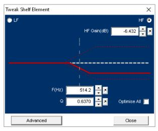
Fig.7 Woofer Shelf Element at 514 Hz
