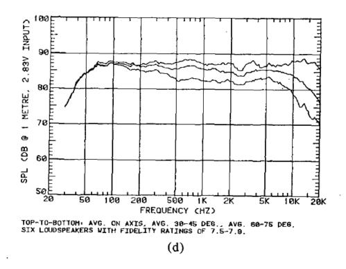
Fig. 2 Amplitude response measurements of loudspeakers with highest fidelity ratings 7.5 to 7.9. (Floyd Toole)
