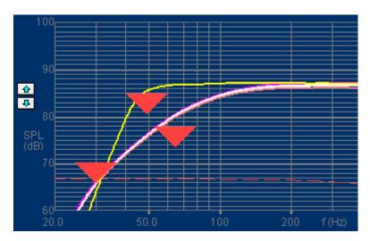
Fig. 19 Low frequency response with Boost (yellow) / without. Red arrows indicating max level
