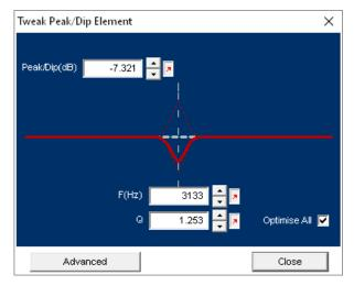
Fig.8 Biquad Peak/Dip Element at 3133 Hz
