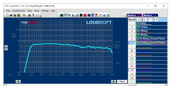
Fig.15 Radiated Sound Power of the final 2-way Loudspeaker calculated over 120deg (+/-60deg)
