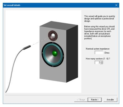
Fig.3 Measuring driver responses on the listening axis
