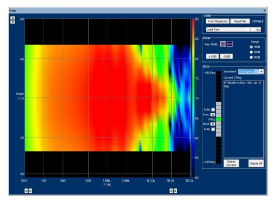
Fig.5 Contour Plot of the Woofer in box
