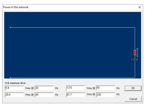
Fig.20 Input Voltages for Xmax at various frequencies
