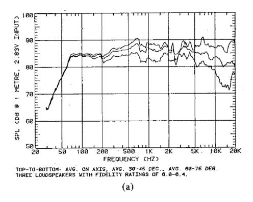
Fig.1 On-axis and two off-axis responses for the worst sounding speakers with fidelity ratings 6.0 - 6.5. (Floyd Toole)
