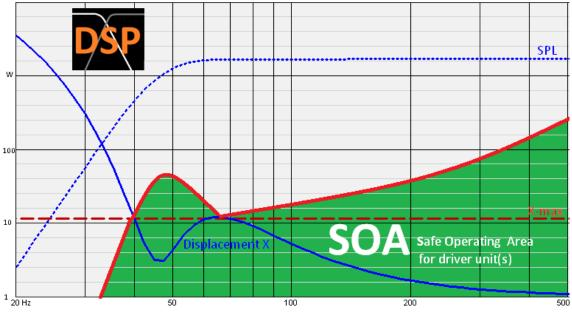
Fig.17 SOA (Safe Operating Area) for driver control with DSP
