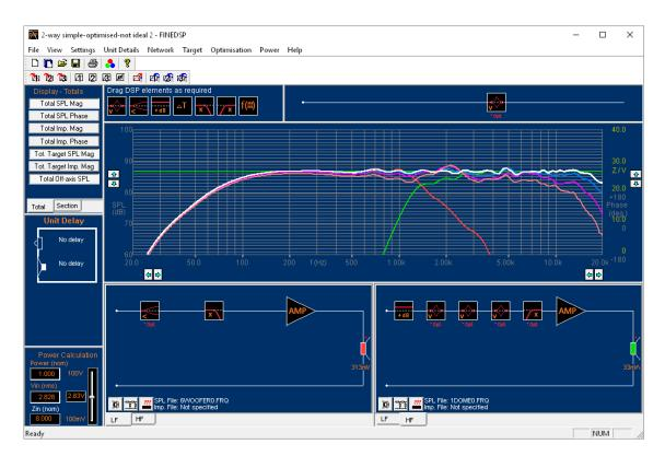
Fig.10 Two way optimized cross over response using only on-axis SPL. Off-axis responses are shown but not used for optimization.
