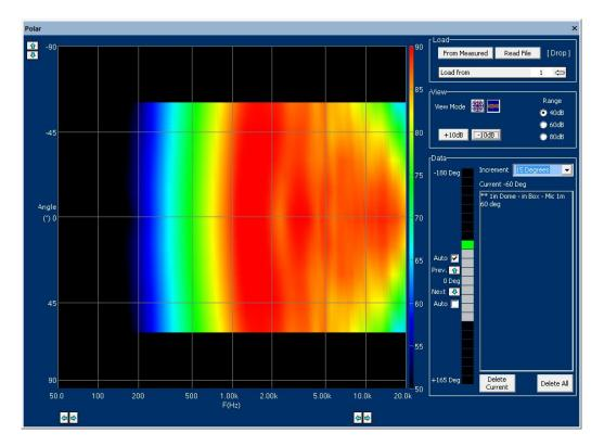
Fig.6 Contour Plot of the Tweeter in box
