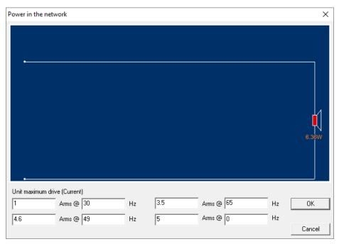
Fig.21 Max Input Current at various frequencies
