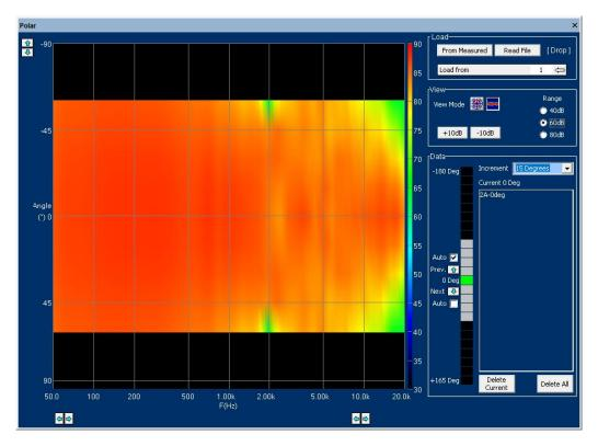
Fig.16 Contour Plot of the final 2-way Loudspeaker calculated for the total angle of 120deg (+/-60deg)
