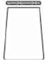
4 Saldobrasatura bordo Braze-welding
