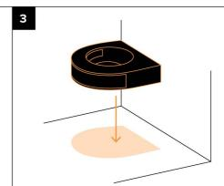
Press bracket firmly onto the countertop for 30 seconds until it is secured.
