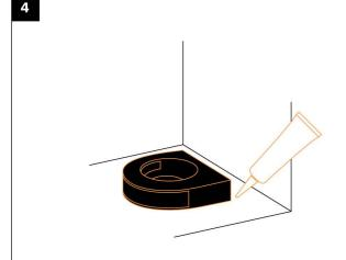
Place a line of adhesive caulk around the bracket to prevent water and grime from getting under the bracket. Wipe away any excess caulk. Wait for 72 hours before inserting the bottles to allow tape to securely set.
