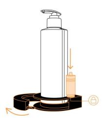
Unscrew magnetic key cap and place key on the lock symbol to unlock the bracket. Open bracket arm and place the bottle inside. Close the arm and remove key. Dispenser is ready to use!
