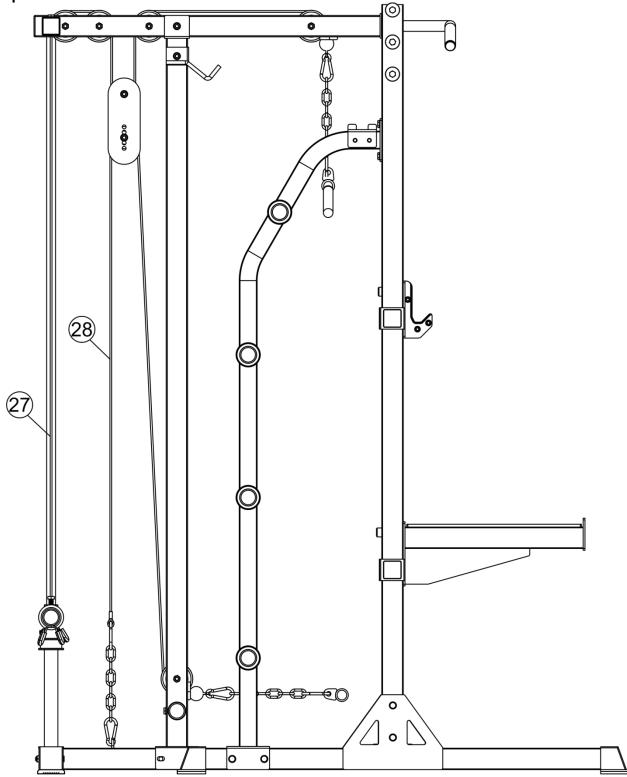
This drawing shows the cable guidance – parts (27) & (28).
