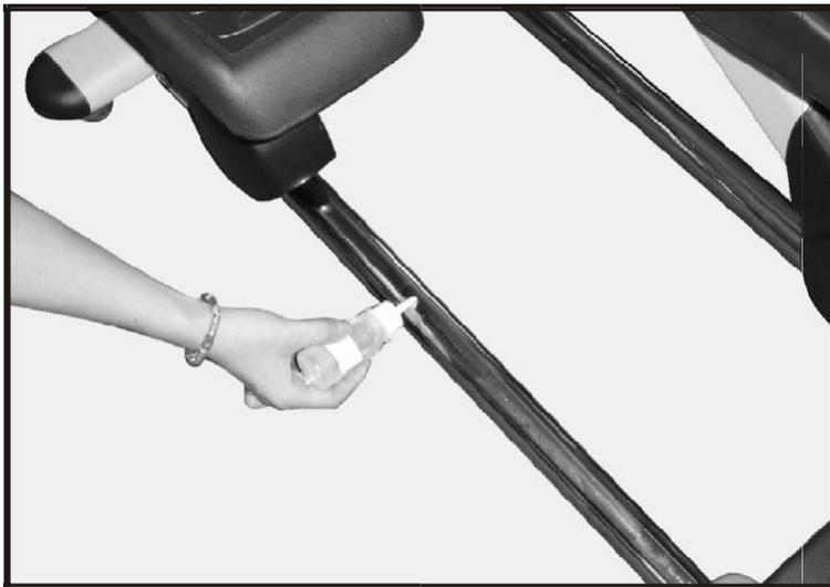
1. Pour 2c.c of the lubricant under the middle of rail. You must be pour lubricant each three months.
