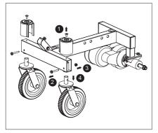
a. Loosen the screws on the wheel cover (No.14) and remove the wheel cover. Then remove M8 bolt (No.13) and nut, and take out the Swivel wheel downwards.
