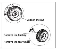
a. Loosen M14 nut (No.16), knock the rear wheel off alternately from left and right with a soft hammer, and remove the flat key (No.4).
