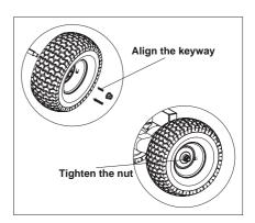
b. Align the keyway surface, knock in the flat key, sleeve the rear wheel on the rear axle with the inflation port outwards, and tighten the M14 nut.
