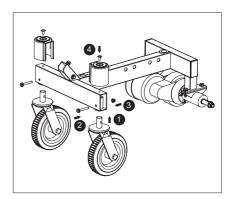
b. Align the fixing shaft of the Swivel wheel with the shaft sleeve in the bracket, insert M8 bolt in alignment with the mounting hole and tighten the nut, and then fix the wheel cover with the screw.
