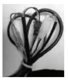
g. Arrange the excess wires in the battery case, secure them with a strap or zip-tie, and put on the battery case cover.
