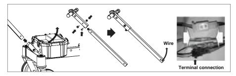
f. Thread the wire into the connecting rod, and then through the front end of the bracket into the battery case. Assemble the handle bar assembly with the connecting rod, and the connecting rod with the bracket, and insert the wire terminal with the terminal of the controller tightly.
