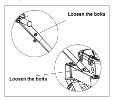
b. Loosen the bolts between the handle bar assembly and the connecting rod, and between the connecting rod and the bracket, pull out the wires and remove the handle bar assembly.
