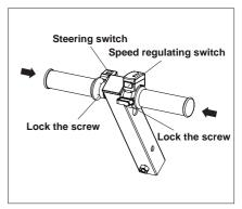
e. Put the new steering switch and speed regulating switch on the handle bar and move them to the appropriate position, lock the lower screw and put on the handle sleeve, thread the wires respectively through the round holes of the square pipes on both sides, and pay attention to protecting the wires and terminals.
