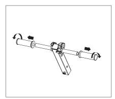
c. Rotate the handle sleeve and forcibly pull it out. Since the handle sleeve is prone to hardening when the ambient temperature is low, it is recommended to cover it with hot and wet cotton cloth before pulling it out.
