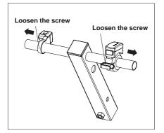
d. Loosen the lock screw at the lower side of the steering switch\speed regulating switch, and move the switch out. Be sure not to use too much force, and pay attention to protecting the wires and terminals.
