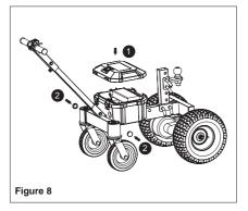
After checking that the wiring harness is connected accurately, replace the case cover and secure the buckle (Step 1); Cover the pipe plug for sealing (Step 2).
