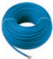
01840.E.B By-me system Bus cable for sound system, 2x0,50 mm 2 , with LSZH sheath, CPR Eca class, suitable for I category cables (U0 = 400 V), blue - 100 m
