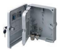
Head terminal, set up for input of 2 cables and 12 filber optics for several dimensions, degree IP65, grey RAL 7035. Supplied with safety locking key. Dimensions: 245x210x65 mm
