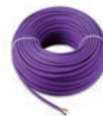
732I.C.100 Due Fili Plus cable for internal/external laying, 2x1 mm 2 twisted conductors, LSZH sheath and insulation, Cca - s1b, d1, a1 class, operating temperature -25/+70°C, insulation degree 600/1000 V, suitable for laying underground in dry ducting or channels with efficient drainage (max. 24 hrs wet), not suitable for laying directly underground, suitable for I category cables (U0 = 400 V) purple, - 100 m bundle
