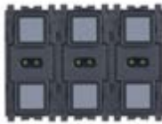
▲21126 6 independent push buttons, 8 non-polarised inputs, 7 solid state outputs for non-polarised contacts, 9-32 VDC power supply - 3 modules. Depth: 22,8 mm
