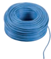
732H.E.100 Due Fili Plus cable for internal laying, 2x1 mm 2 twisted conductors, PVC sheath, CPR Eca class, operating temperature -25/+70 °C, not suitable for running through underground channels, suitable for I category cables (U0 = 400 V), blue - 100 m bundle
