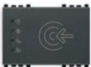
20457 Transponder card reader for installation outside rooms, KNX standard, 2 NO 4 A 24 V~ relay outputs, 2 inputs, power supply 12-24 V~ 50/60 Hz and 12-24 Vdc (SELV) - 3 modules. Supplied without transponder card. Depth: 37 mm
