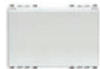
20453.N Transponder card reader with vertical pocket for installation inside rooms, KNX standard, 2 NO 4 A 24 V~ relay outputs, 2 inputs, power supply 12-24 V~ 50/60 Hz and 12-24 Vdc (SELV) - 3 modules. Depth: 37 mm
