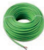
732I.E.100 Due Fili Plus cable for internal/external laying, 2x1 mm 2 twisted conductors, LSZH sheath and insulation, CPR Eca class, operating temperature -25/+70°C, insulation degree 600/1000 V, suitable for laying underground in dry ducting or channels with efficient drainage (max. 24 hrs wet), not suitable for laying directly underground, suitable for I category cables (U0 = 400 V), green - 100 m bundle
