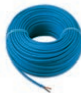
01840.E.B Cable for sound system, 2x0,50 mm 2 , with LSZH sheath, CPR Eca class, suitable for I category cables (U0 = 400 V), blue - 100 m
