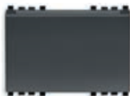
20453 Transponder card reader with vertical pocket for installation inside rooms, KNX standard, 2 NO 4 A 24 V~ relay outputs, 2 inputs, power supply 12-24 V~ 50/60 Hz and 12-24 Vdc (SELV) - 3 modules. Depth: 37 mm
