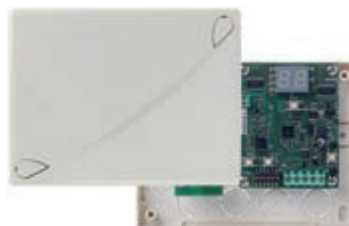
01729 Two-way 868 MHz radiofrequency interface
