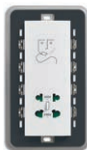
20291.B 6 230 V~ 50/60 Hz, with 20 VA isolating transformer, 230 V~ and 120 V~ outputs. Depth: 41 mm
