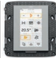
21848.1.BN Color touch screen, 4,3", Full Flat, for the control, 1 temperature sensor input, with built-in mounting frame for installation in 8-module mounting box. Depth: 50,4 mm
