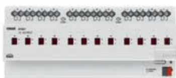
01521 Actuator with 12 10 A 250 V~ 50/60 Hz relay outputs for fluorescent lamps, KNX standard, 12 x 17,5 mm modules
