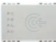
20457.N Transponder card reader for installation outside rooms, KNX standard, 2 NO 4 A 24 V~ relay outputs, 2 inputs, power supply 12-24 V~ 50/60 Hz and 12-24 Vdc (SELV) - 3 modules. Supplied without transponder card. Depth: 37 mm
