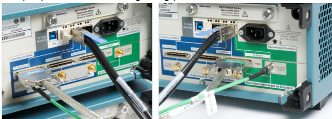
UltraSync connection on instrument with Master role
