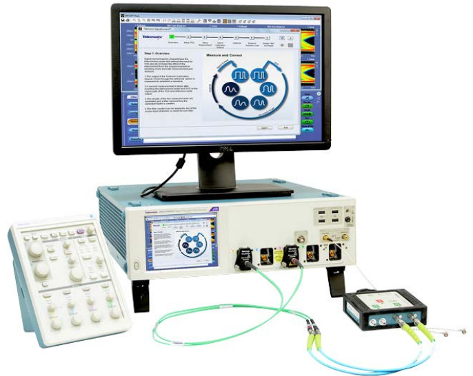
SignalCorrect allows quick characterization of cables, fixtures and other types of interconnects using the TCS70902 fast step source and the response captured on a DPO7000SX Series real-time oscilloscope.
