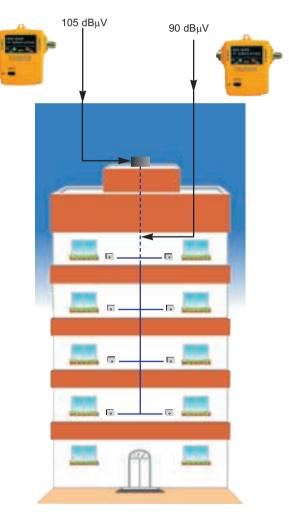
6 SATELLITE IF BAND EQUALISATION It generates three signals in the satellite band. With a spectrum analyser the adjustment of the SLOPE-TILT can be easily made. It also generates a signal in the UHF band.
