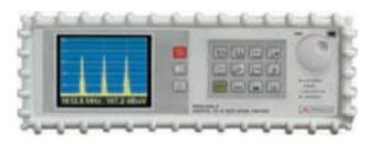
The **PROLINK-4** has a function (SAT IF TEST) which automatically stores the exact levels for each carrier at the Headend and reads the value of attenuation calibrated at each frequency.
