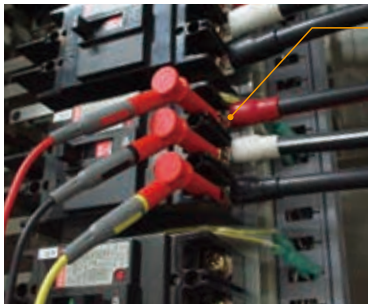
Magnetic design (diameter: 11 mm)
