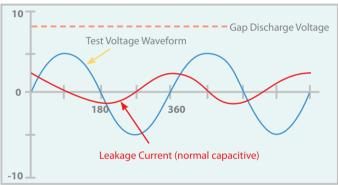
Leakage Current (normal capacitive)
