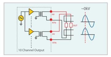
Figure 1: Unsynchronized Output
