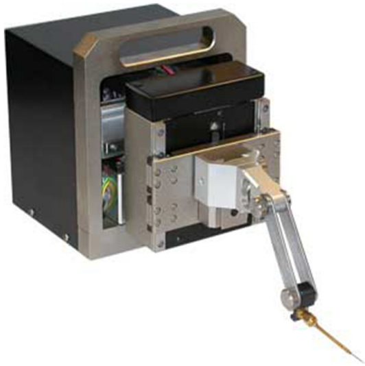
SAM Submicron Automated Manipulator
