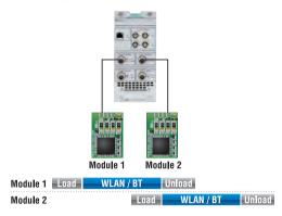
One TRX Test Module can be used to measure WLAN 802.11b/g/a/n/p/ac, 11ac (Wave 2), 11ax and Bluetooth v5 modules.
