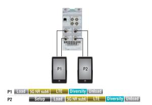
Two TRX Test Modules can be used to measure multiple wireless technologies in one smartphone.
