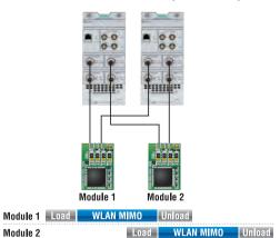
Using two TRX Test Modules supports True MIMO measurement of WLAN 802.11n and 11ac 2×2 MIMO modules.
