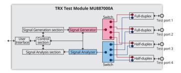
The MU887001A has four duplex RF connectors.
