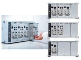
★1: Test modules cannot be hot-swapped with the power on.
