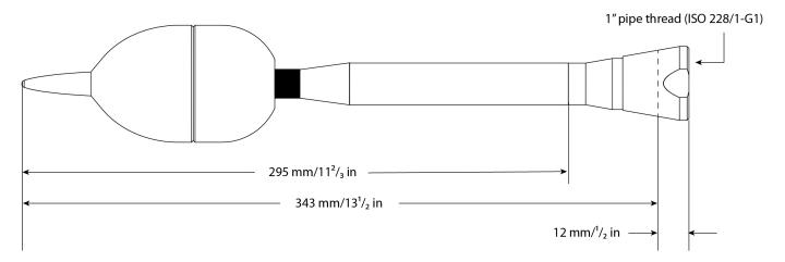
When mounted on a pipe: 343 mm / 131/2 in above the top of the pipe.
