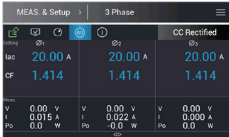
Regenerative AC Load in 3-Phase Mode
