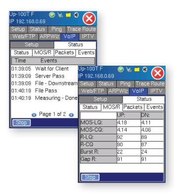
**VoIP Expert** – Generates industry standard wave files to verify MOS and R-factor values of upstream and downstream paths and includes QoS measurements such as packet jitter, packet loss, and delay. Compatible with all VeEX testers including VX1000 VoIP server software.
