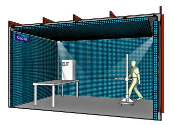
The Chronos 1F ISO is designed to perform emission and immunity tests on automotive components. The design of the structure is optimised for maximum performances, in minimum space. The shielding and its pyramidal absorbers are manufactured by SIEPEL.
