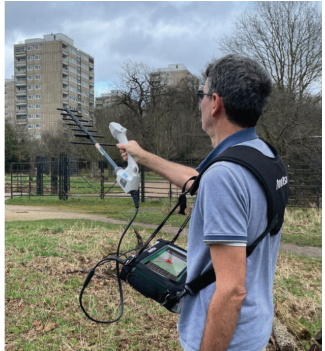
A Directional Antenna Coupled to the Interference Hunter MA2700A Provides Rapid Geolocation of RF Sources
