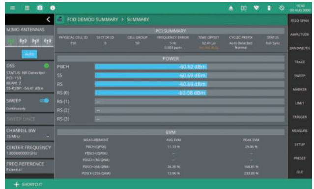
LTE Results Summary with DSS Detection Result Displayed in the Status Panel
