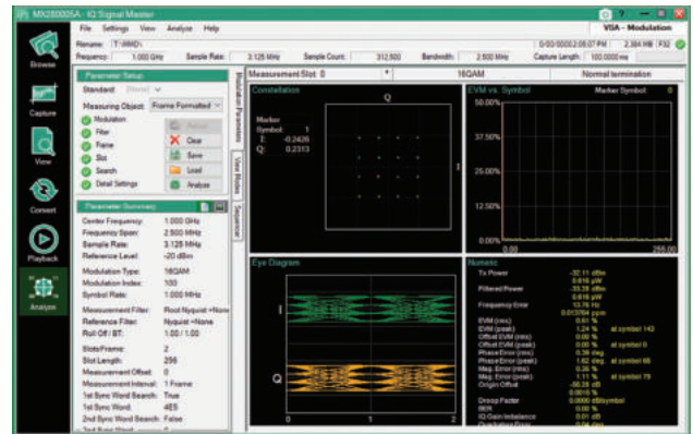
MX280005A Single Screen Multiple Results Vector Signal Modulation Windows
