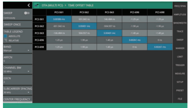
Time Offset Table Shows the Relative Time Offset Between Signals Arriving From All gNB
