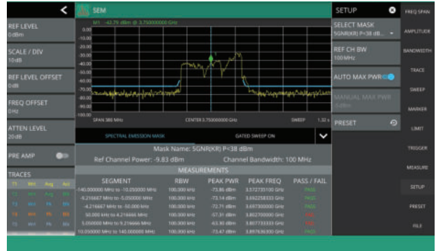
OTA SEM Measurement on a 5G NR Transmission with Pass/Fail Results
