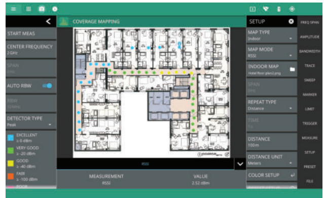
Typical Result Screen for Indoor Coverage Mapping
