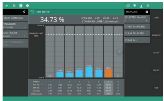
EMF Meter Displays Percentage of ICNIRP Limit over Time at Up to 16 Positions at Any Given Site
