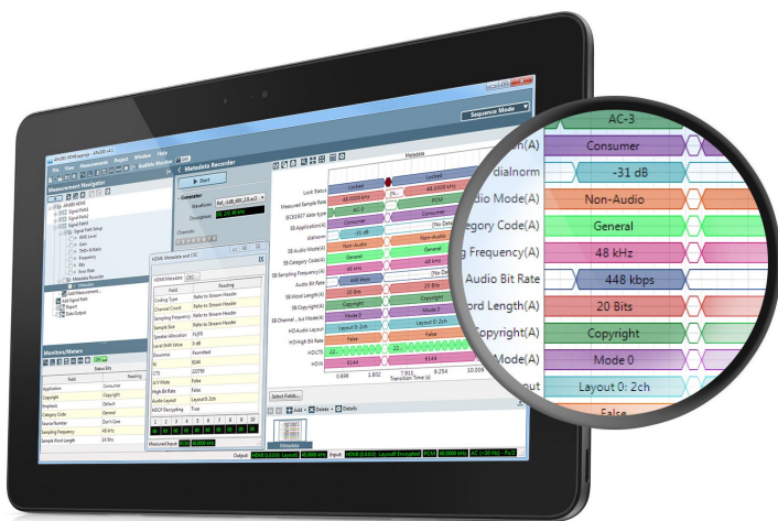
APx500 Measurement Software metadata recorder tracking HDMI metadata changes.
