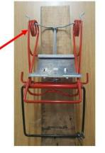
Formed catch holds lower rung, stopping slipping, and fixing the trap firmly in place.
