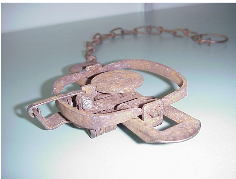
Figure 4. Traps should be set fine (i.e. trap dog just under the trigger latch) with the trigger plate at the same level as the jaws.
