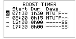
Alternatively the eSense input can be used to active the boost whenever the economy tariff rate electricity is available, regardless of boost times (option 2). To do this, the eSense Input option in the Advanced menu should be set to Boost. When using this option, the Boost Timer is not needed.
