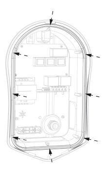
Ensure O-ring is present and sits neatly into its channel.
