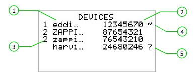
All linked devices  $\bigcirc{1}$  are listed in the DEVICES screen, the device shown in CAPITAL letters is the device currently being viewed. The serial number of each device is shown on the right  $\bigcirc{2}$
