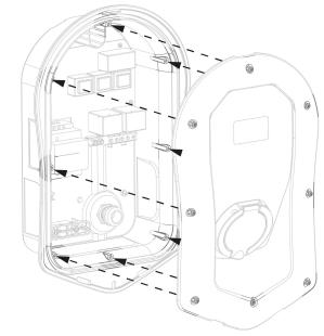
Offer cover to the enclosure ensuring all cables are neatly inside the unit.
