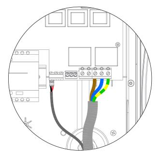
For single phase installations where 1 or 2 external / hardwiring an external CT please follow the above additional CT's are required, please follow the above diagram to connect the CT's using the extra 2 CT terminals in the same way if required.
