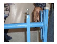
4. Mount Pot Support on the stand after inserting the Reflector Cradle support members. Now tighten all the bolts which were loosely fitted in earlier steps.
