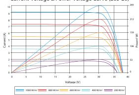
Excellent performance under weak light conditions: at an irradiation intensity of 200 W/m<sup>2</sup> (AM 1.5, 25 °C), **96.5%** or higher of the STC efficiency (1000 W/m<sup>2</sup>) is achieved
