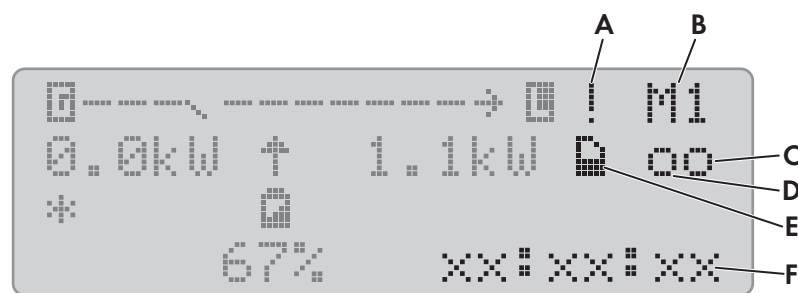
Figure 8: Status of the Sunny Island inverter (example)
