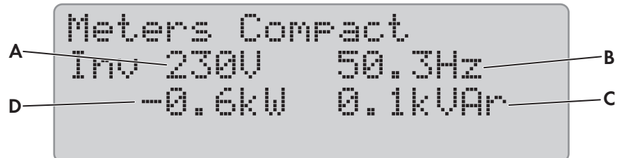
Figure 16: Overview of the menu Meters Compact for the AC measured values of the Sunny Island inverter
