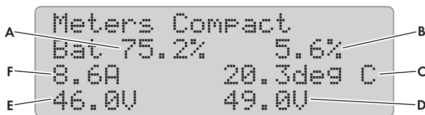
Figure 15: Overview of the menu Meters Compact for the battery
