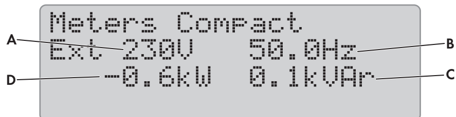
Figure 17: Overview of the menu Meters Compact for the generator or the battery backup grid
