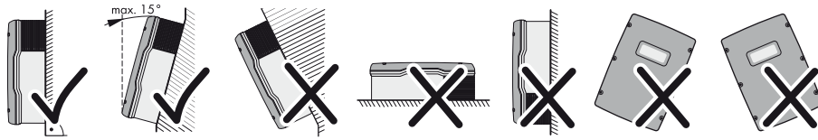
Figure 5: Permitted and prohibited mounting positions
