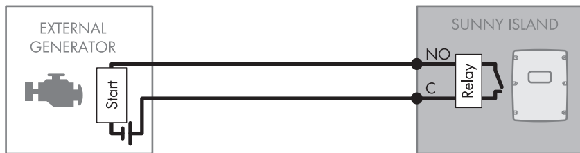
Figure 11: Connecting the Generator Control to Sunny Island
