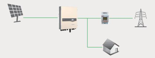
If the household loads and the PV generation curve are well matched, battery module may not be required, the SH5K hybrid inverter and meter could be used as a "Zero-export" system. In this system, the inverter output will be derated to ensure the feed-in power be zero when a feed-in power above zero is detected by the meter.
