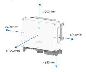
\* The distance can be shortened to 200mm according to onsite conditions. In case the distance is less than 600mm, move the inverter from the mounting-bracket or wall before maintaining fans.
