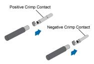
**step 3** Lead the cable through cable gland, and insert into the insulator until it snaps into place. Gently pull the cable backward to ensure firm connection. Tighten the cable gland and the insulator (torque 2.5 N.m to 3 N.m).
