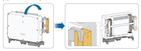
**step 7** Fix the inverter with two M6  $\times$  65 screws.
