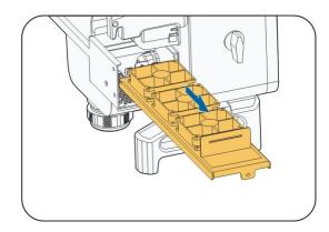
**step 5** Reinstall the fan back to the inverter in reverse order and restart the inverter.
