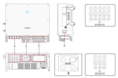
figure 5-1 Wiring terminals
