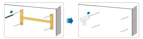
**step 3** Insert the expansion bolts into the holes and secure them with a rubber hammer. Fasten the nut with a wrench to expand the bolt. Remove the nut, spring washer, and flat washer, and store them properly.
