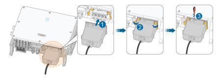
**step 8** Gently pull the cable backwards to ensure firm connection, and fasten the swivel nut clockwise.
