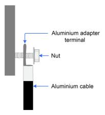
figure 5-3 Aluminium cable terminal connection sequence
