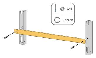
**step 2** Level the assembled mounting-bracket by using the level, and mark the positions for drilling holes on the installation site.
