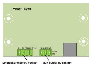
DO terminal (fault output dry contact): the relay can be set to fault alarm output, and
