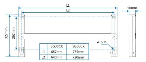
figure 4-1 Dimensions of mounting-bracket
