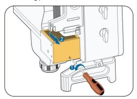
**step 3** Press the hump of the latch hook, unplug the cable connection joint outwards, and loosen the screw on the fan holder.
