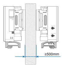
• Install the inverter at an appropriate height for ease of viewing LED indicators and operating switches.
