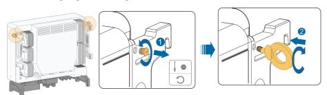
**step 2** Lead the sling through the two lifting rings and fasten the tie-down strap.
