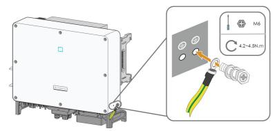
**step 3** Apply paint to the grounding terminal to ensure corrosion resistance.
