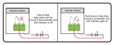
figure 5-5 Normal open contact
