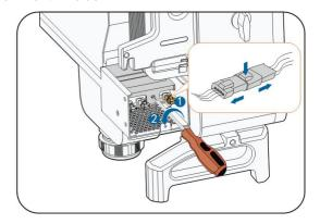
**step 4** Pull out the fan module, clean the fans with soft brush or vacuum cleaner, and replace them when necessary.
