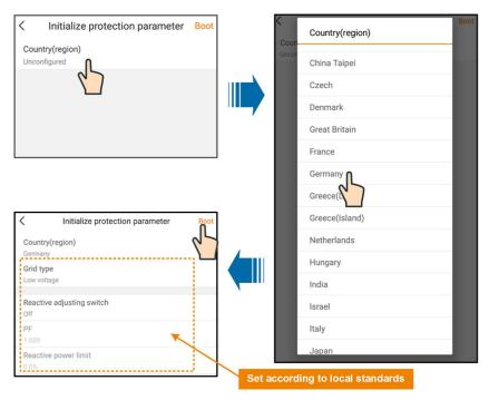
figure 7-3 Initialization protection parameter
