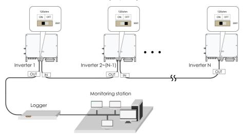
figure 5-4 Configuration of dip switch (N≥15)
