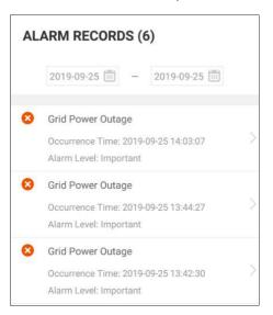
figure 7-8 Fault and alarm records
