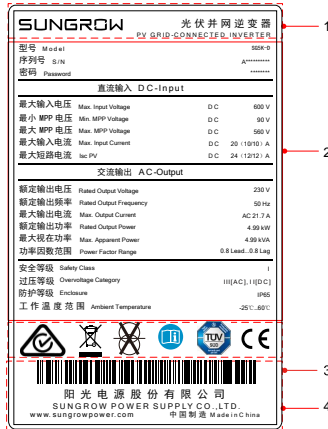
Fig. 3-2 Nameplate of Inverter
