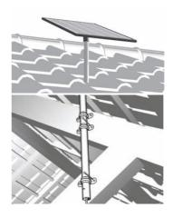
The Solar Panel is designed to be mounted on a rigid pole. An aluminium or gal. pipe of 26 mm diameter is ideal, but a thick PVC pipe is acceptable. The pole should be mounted on the rooftop, clamped or tied to the truss of the roof. If you cannot mount it there, you can also nail the pole on
