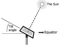
To adjust the angle of the solar panel, loosen the 4 "Allen" (socket head) screws with a suitable 3mm "Allen" key. Loosen each screw by approximately 2 turns and the angled swivel
