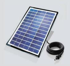
LEC 150 stands for Light to Electricity Converter and can be used for charging Sundaya Ulitium lamps but also all other Sundaya products that can accept charge from 16 to 25VDC charge voltage range. The LEC is made of very durable and high strength material to ensure a very long life in all weather conditions. The LEC is delivered complete with 500cm cable and pole-mountable support with angle ajustable Swivel.
