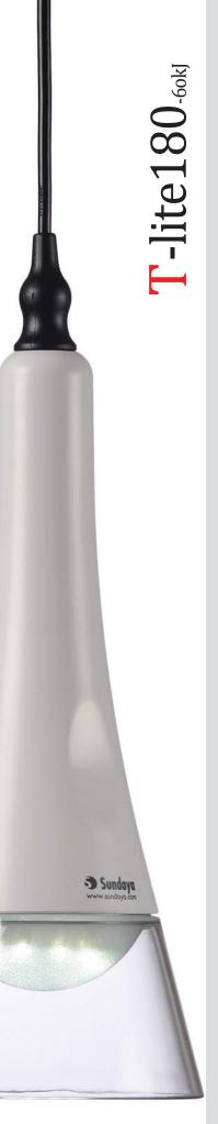
The T-lite 180 is a lamp based on ultra efficient Light Emitting Diode Technology with built in Lithium Energy Storage Pack and energy management electronics. The T-lite can deliver up to 180 Lumens of Light output to a maximum of 7,5 hours on a full Charge or a Maximum of 75 hours at a lightoutput of 15 Lumens. The T-lite is operated through a Touch-Switch with dimming function. The T-lite can be used as a hanging, or standing Lamp but also as a torchlight with an ergonomically designed handle.
