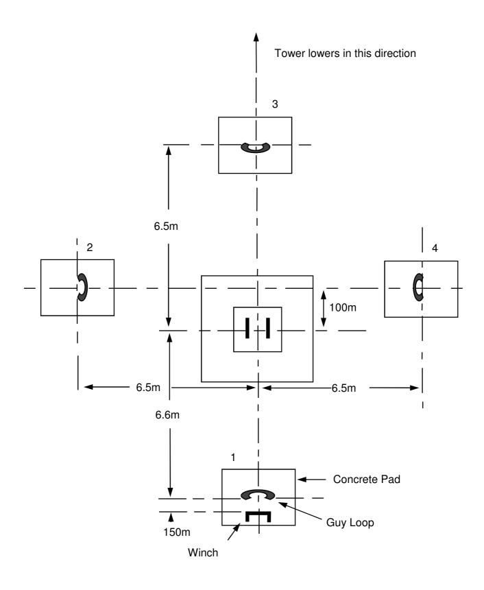
Fig 2. Plan view of 13m Tower Foundations not to scale
