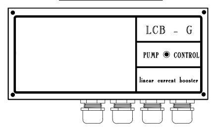
The "LCB - G" pump controller is a high quality DC power converter designed as an interface between a DC (Solar)-Pump (e.g. SHURflo 9300) and a DC power source, like solar panels, wind generators, batteries etc.. The main function of this controller is to maximize the daily water output while providing protection for the pump. The controller can be used in 12V and 24V systems.
