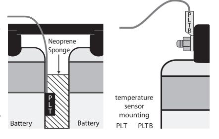
Fig. 7.4.3A - Attaching a Temperature Sensor to a battery
