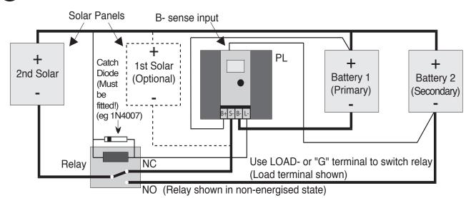
Fig. 7.5.4A - Second Battery Control
