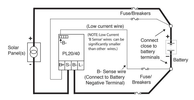
Fig. 7.5.3A - Battery Sense Input
