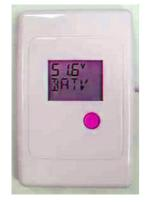
The PLM remote monitor is a device which allows remote user access to a PL series charge controller. It shows exactly the same information as the PL screen and the PLM button behaves in exactly the same way as the button on the PL.. This means you can use the PLM for everything you would normally do at the PL itself. only in а more
