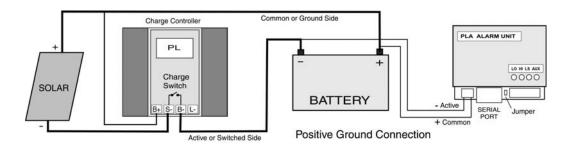
(If the PLA is to be used on its own, then it does not matter which way the power is connected to it. It will work with voltages of either polarity. When first connected, the PLA assumes a positive ground connection. If it is actually connected as negative ground, it will automatically swap to negative ground after 20 seconds.)
