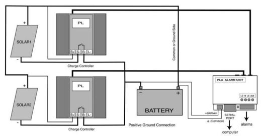
Connection of a two PL controller system with a PLA
