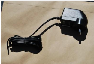
240 to 12-volt Transformer
