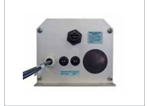
Figure 4: Bottom of controller with prewired plugs
