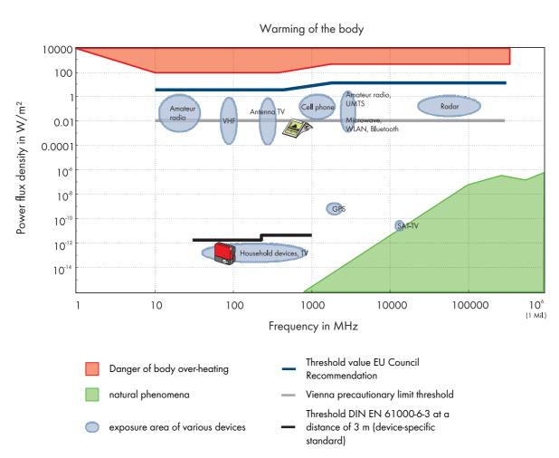
This compilation is not absolutely accurate or exhaustive, rather is based on illustrative measured and empirical values, e.g. from literature (LfAS "Electromagnetic fields in the work place", G. Bopp (ISE) "Do PV systems cause electro-smog?"). In exceptions, the values can also fall above or below the marked area.
