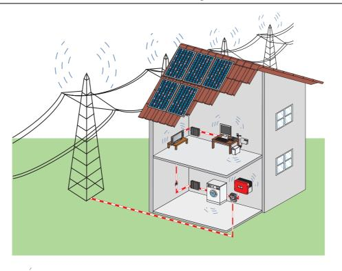
L<sup>1</sup>, Radiation based disturbances — Cable based disturbances
